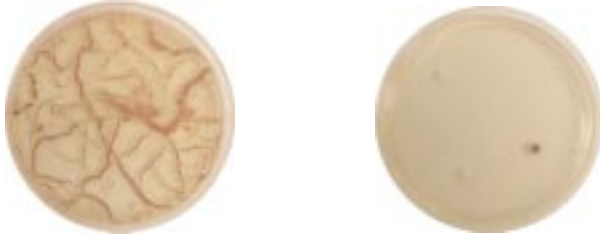
Before and after bacteria samples application of BOS unit to commercial dumpster compactor
