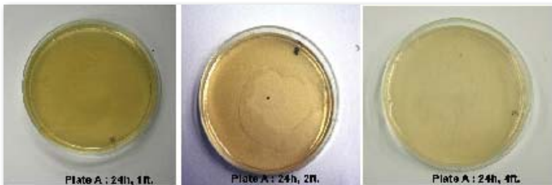
Figure 3 Number of Microbial Colonies Produced in the Control Set AFTER Any Treatment of indoor Air with the Air Purifier (Measured at 1 ft., 2ft., and 4 ft.)
